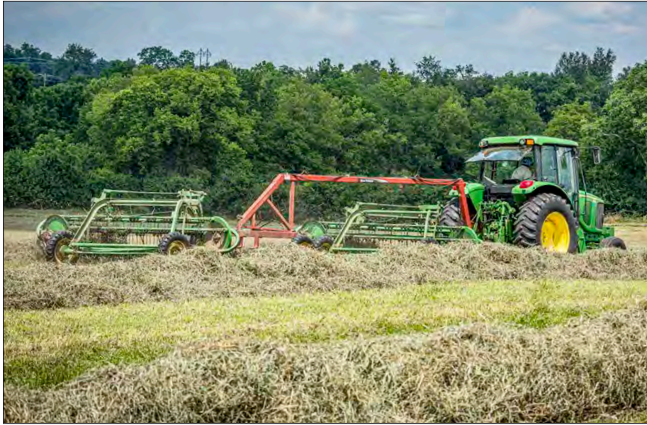
Using wide raking equipment like this tandem bar rake will help to minimize wheel traffic across hayfields.
